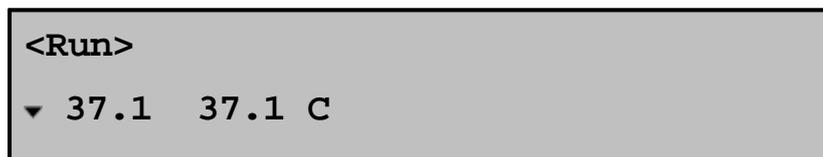
To exit standby mode, press the **Enter** key on the front panel. The incubator will then begin to control the chamber temperatures and gas flow.
